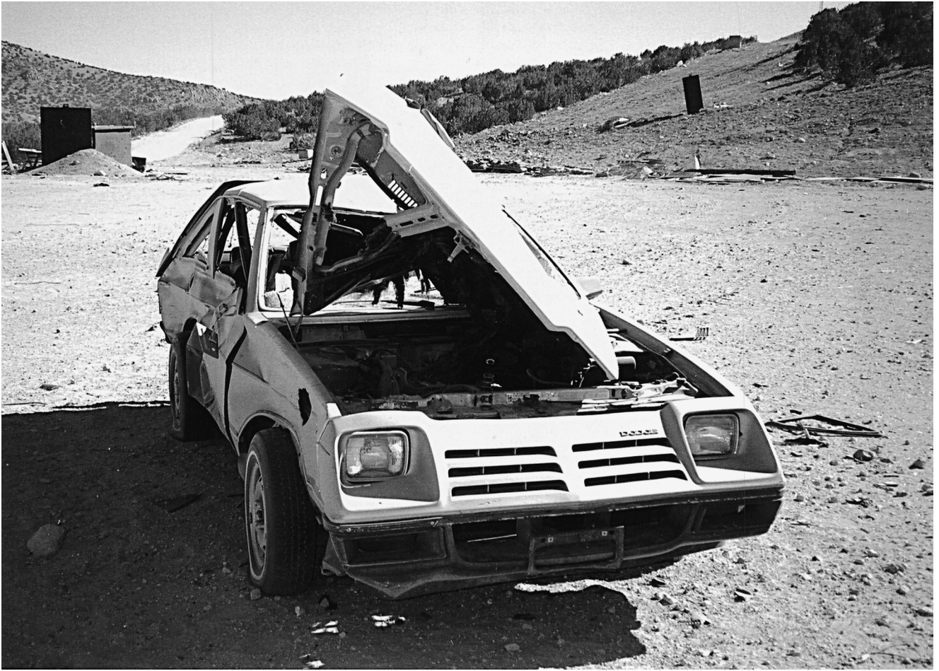
FIG. 19—Damaged Dodge positioned 30 m from 2268 kg charge.
