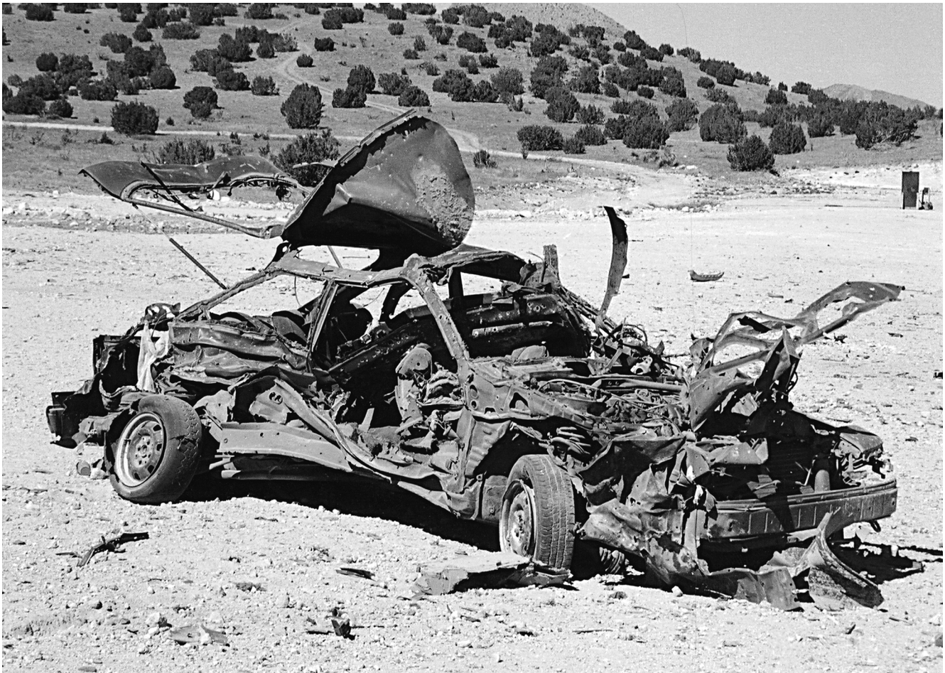
FIG. 18—Damaged Toyota Celica positioned 15 m from 2268 kg charge.
