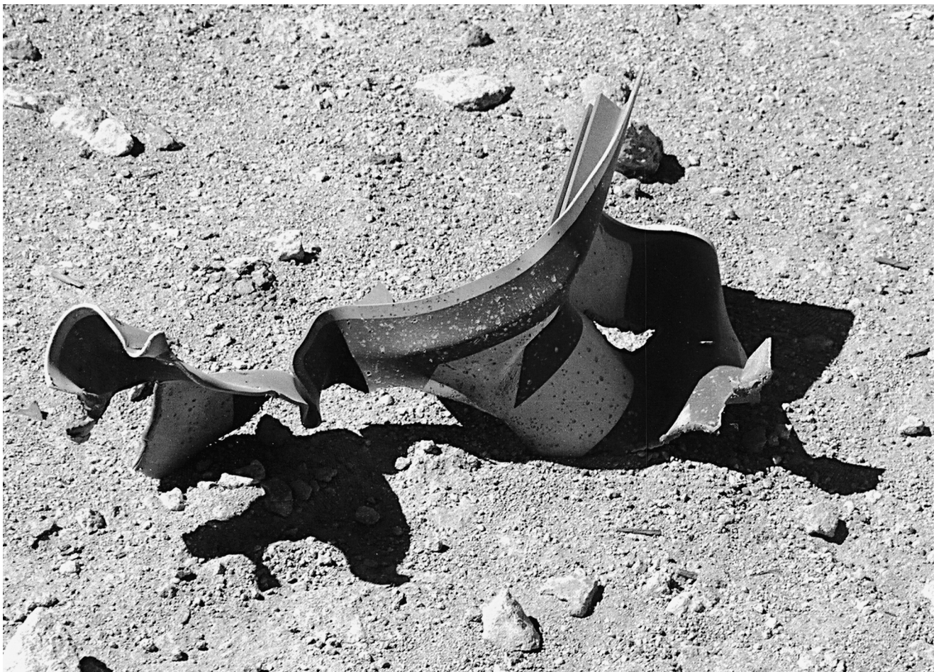
FIG. 16—Road sign showing typical damage at 8 m from 2268 kg charge.
