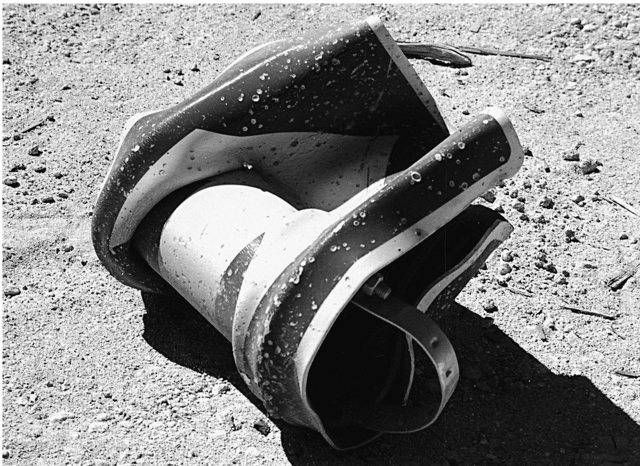
FIG. 17—Road sign showing typical damage at 15 m from 2268 kg charge.
